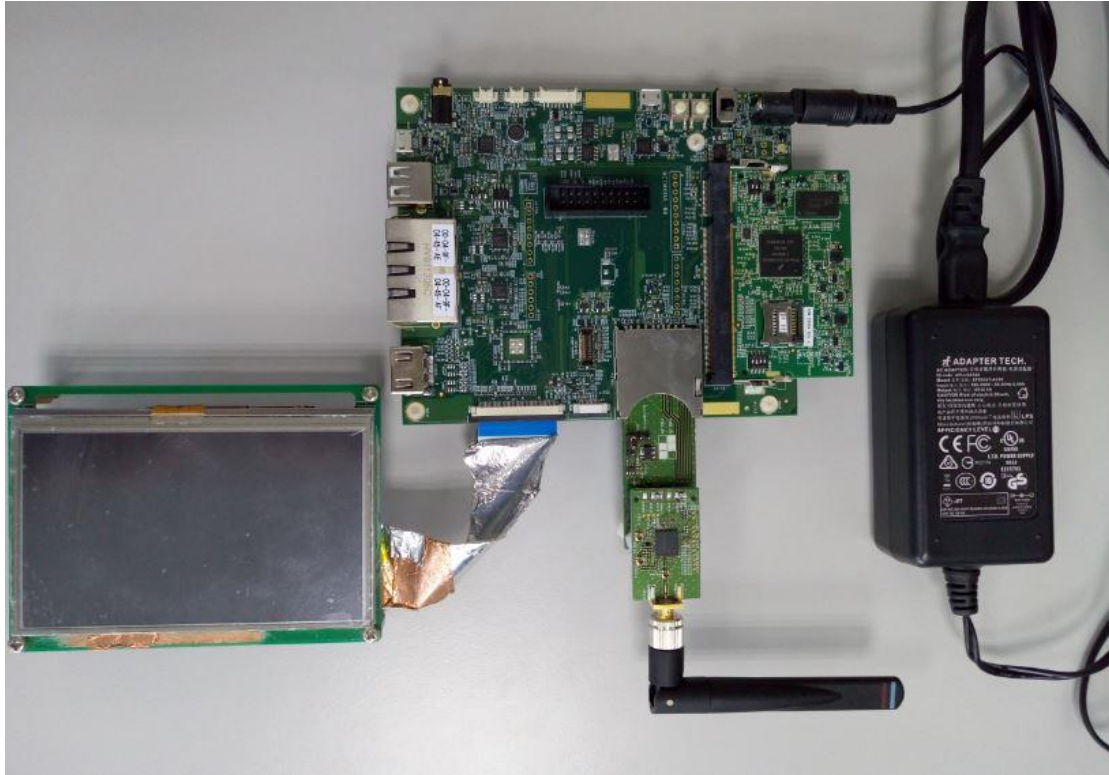
Figure 3. Overview of the i.MX 6ULL EVK board connection
